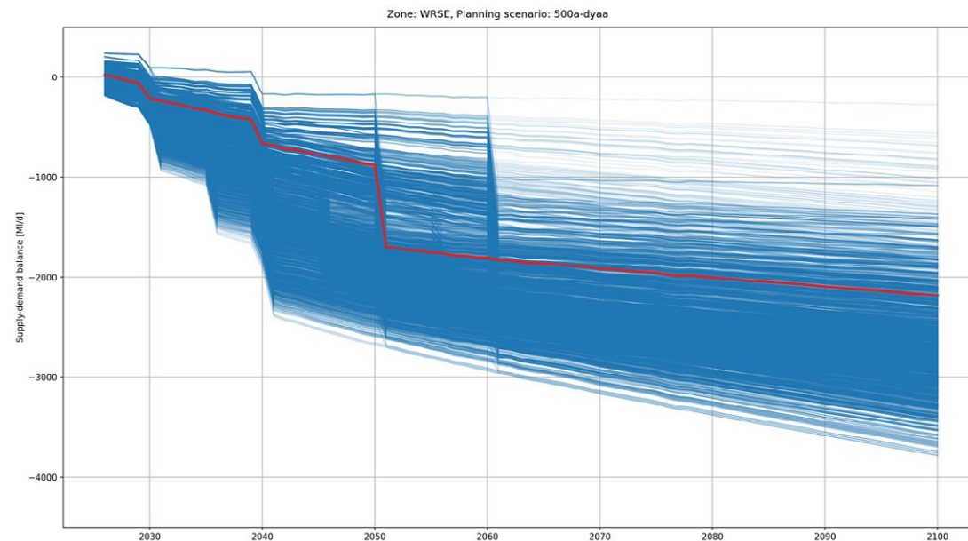
Figure 5.24: The range of baseline supply-demand balances for WRSE region under a 1:500 DYAA scenario
